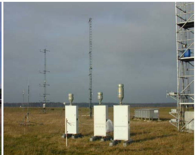
Fig. 4: Melpitz site, view to north, in the foreground DIGITEL-filter-sampler for particles PM_1 , PM_{2.5} and PM_{10}
