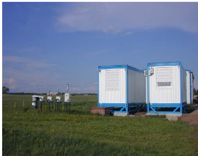
Fig. 3: Melpitz site, view to east, with wet only Sampler, Partisol "2000" filter-sampler and containers for data acquisition and special sampling technique
